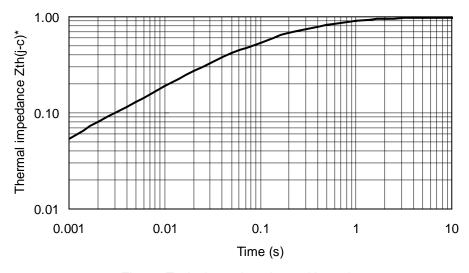
Fig.2-1 Typical transient thermal impedance
