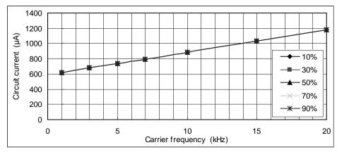
Fig.4-3 I<sub>DB</sub> vs. Carrier frequency for PS22A72
