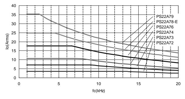
Fig.3-21 Effective current-carrier frequency characteristic
