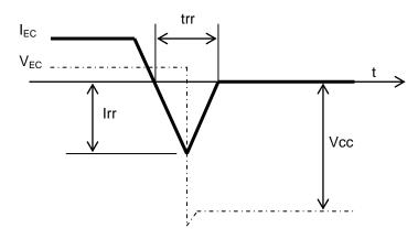
Fig.3-20 Ideal FWDi recovery characteristics curve
