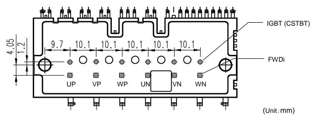
Fig.2-21 Power chip position
