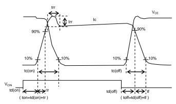
Fig.2-2 Switching time definition
