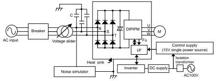
Fig.3-23 Noise withstand capability evaluation circuit
