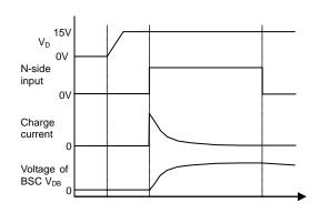
Fig.4-10 Example of waveform by one charging pulse
