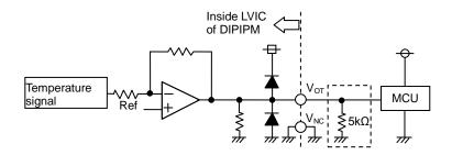
Fig.2-16 V<sub>OT</sub> output circuit in the case of detecting low temperature
