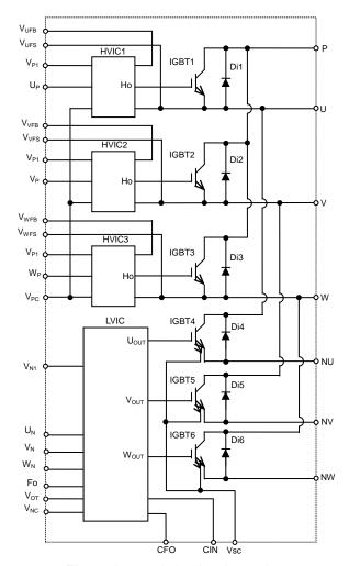
Fig.1-3 Internal circuit schematic
