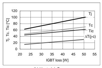
(a) Heat sink A (b) Heat sink B Fig.2-12 IGBT loss vs. Tj, Tc, Tic(Ta=25°C, Typical)
