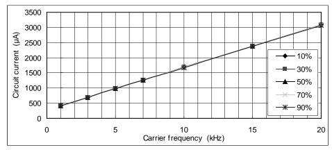
Fig.4-8 I<sub>DB</sub> vs. Carrier frequency for PS22A79
