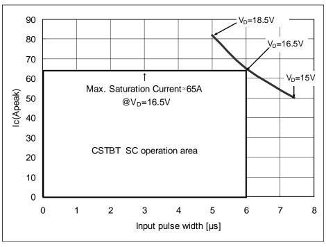
Fig.3-13 PS22A72 typical SCSOA curve
