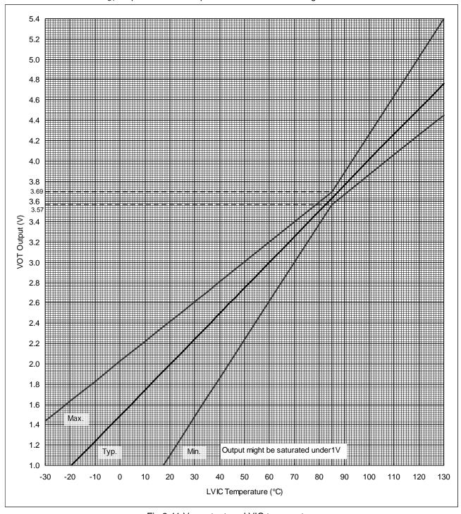
Fig.2-11  $V_{\text{OT}}$  output vs. LVIC temperature
