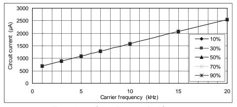
Fig.4-6  $I_{DB}$  vs. Carrier frequency for PS22A76
