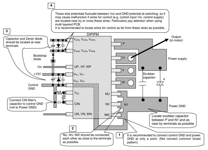
Fig.3-10 Precaution for wiring on PCB
