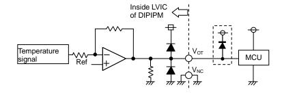
Fig.2-17 V<sub>OT</sub> output circuit in the case of using with low voltage controller
