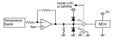
Fig.2-15 Inner circuit of V<sub>OT</sub> terminal
