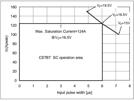
Fig.3-14 PS22A73 typical SCSOA curve
