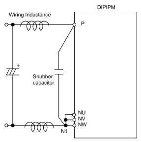
Fig.3-8 Recommended snubber circuit position
