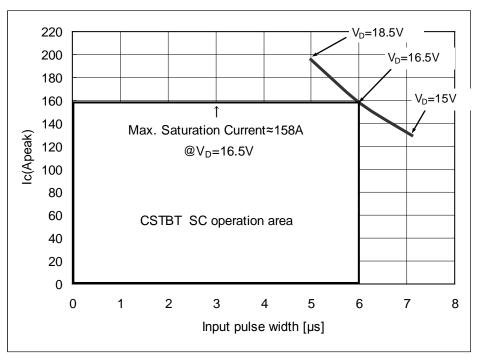
Fig.3-15 PS22A74 typical SCSOA curve
