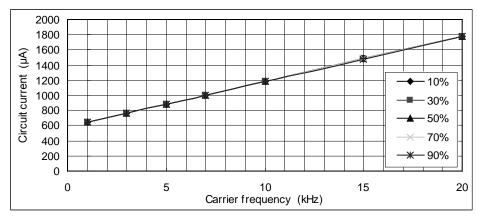
Fig.4-5 I<sub>DB</sub> vs. Carrier frequency for PS22A74
