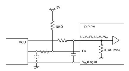
Fig.3-5 Control input connection
