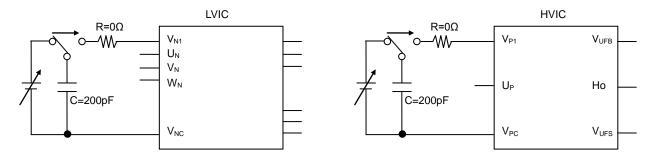
Fig.3-25 Surge test circuit example(V<sub>N1</sub> terminal)
