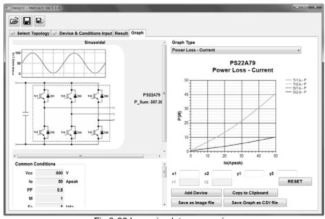
Fig.3-22 Loss simulator screen image
