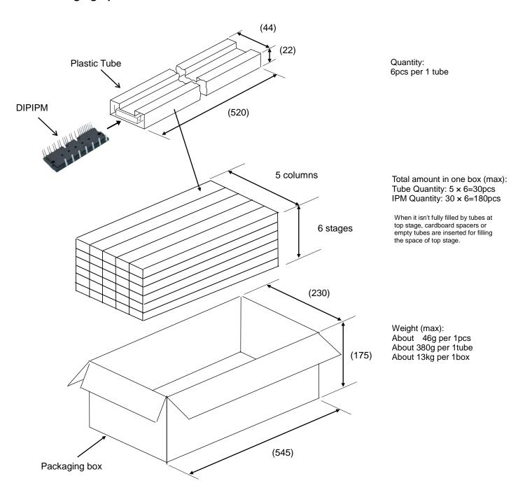
Spacers are inserted into the top and bottom of the box. If there is some space on top of the box, additional buffer materials are also inserted.
