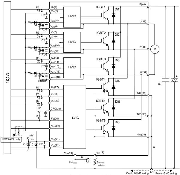
Fig.3-2 Interface circuit example (Direct coupling)
