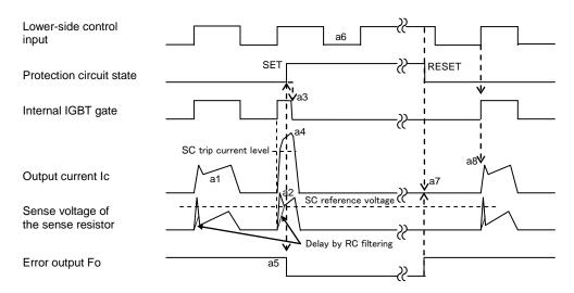
Fig.2-6 SC protection timing chart
