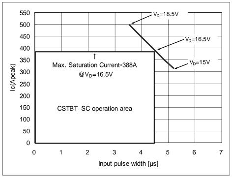
Fig.3-18 PS22A79 typical SCSOA curve
