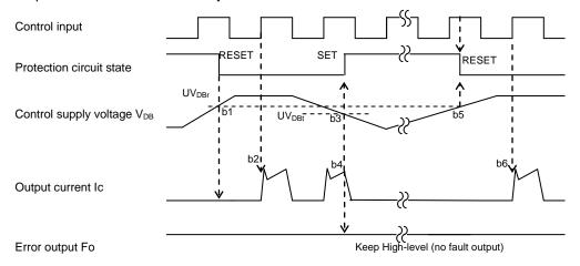
Fig.2-9 Timing Chart of P-side UV protection
