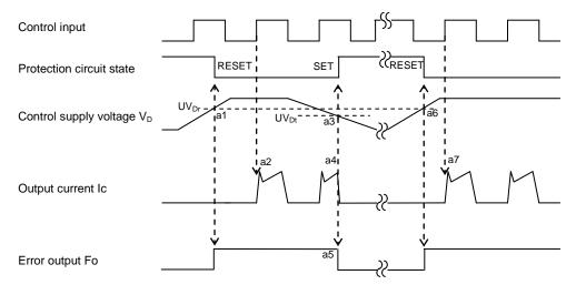
Fig.2-8 Timing chart of N-side UV protection
