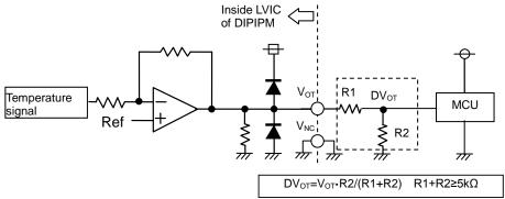
Fig.2-18 V<sub>OT</sub> output circuit in the case with high protection level
