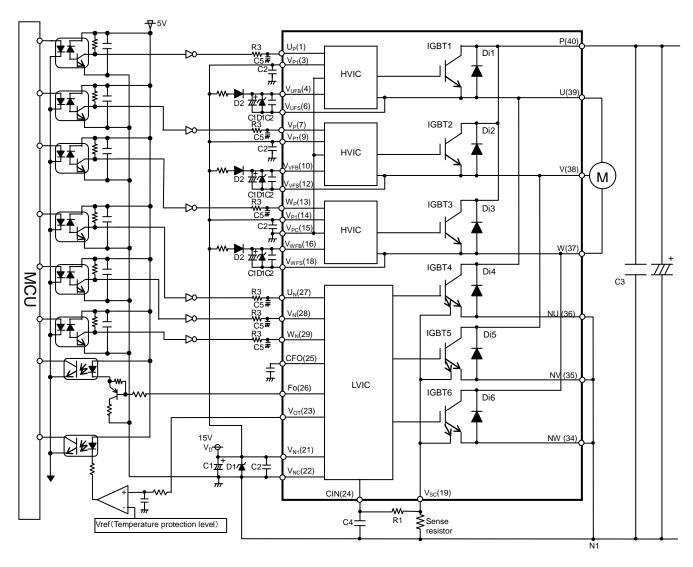
Fig.3-3 Interface circuit example with opto-coupler
