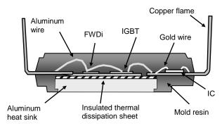
Fig.1-2 Internal cross-section structure
