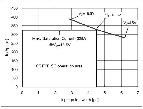
Fig.3-16 PS22A76 typical SCSOA curve
