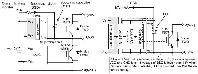
Fig.4-1 Bootstrap Circuit Diagram
