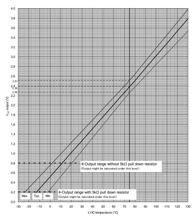
Fig.2-19 V<sub>OT</sub> output vs. LVIC temperature
