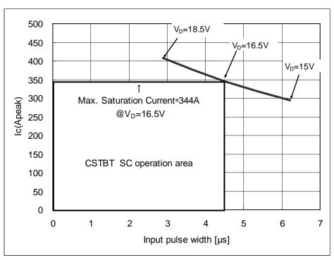
Fig.3-17 PS22A78-E typical SCSOA curve
