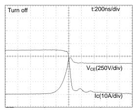
Conditions:  $V_{CC}$ =600V,  $V_D$ = $V_D$ =15V, Tj=125°C, Ic=35A, Inductive load half-bridge circuit Fig.2-4 Typical switching waveform (PS22A78-E)
