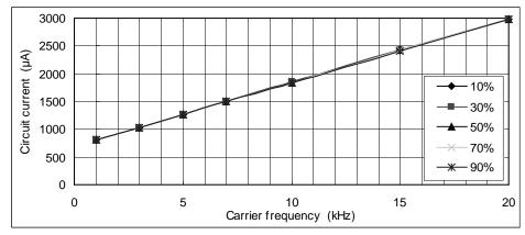
Fig.4-7 I<sub>DB</sub> vs. Carrier frequency for PS22A78-E
